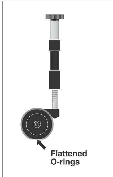
Figure 5-6. Standard O-Ring Gate
