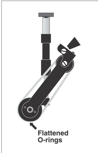
Figure 5-5. Advancing O-Ring Gate
