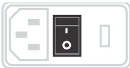
Turn the feeder power On by pushing the horizontal line (—) at the Power On/Off rocker switch.
